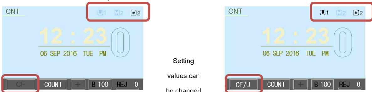
Setting values can be changed by pressing the LEVEL key.
