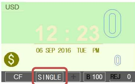
**ORIENT-SORT MODE** (By pressing MODE + LEVEL key)
