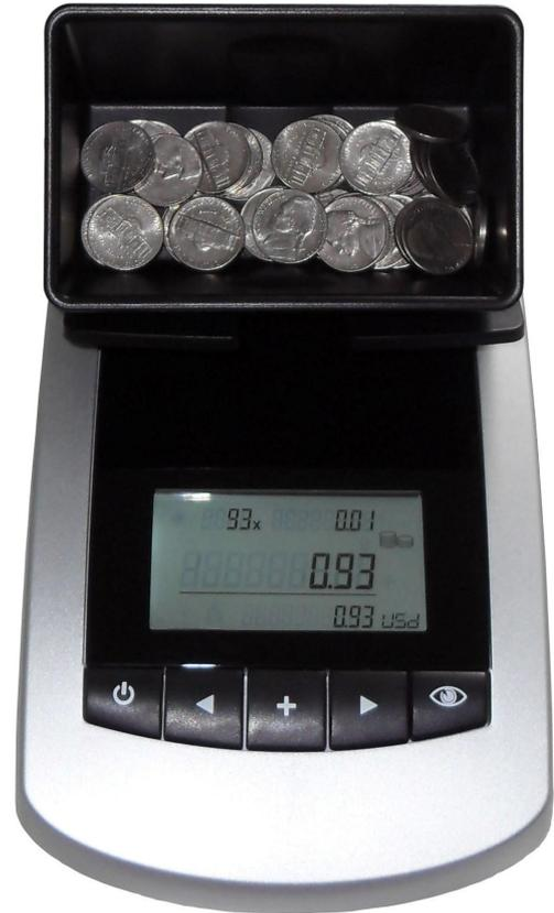
**The MCS 1000** is an all-round machine that will help you count your coins and banknotes in a few minutes! The MCS 1000 features counting for 3 default currencies while other currency tables can be loaded into the machine via its built-in USB port. The counting results are displayed on a large back-lit LCD screen and can be printed instantly via a receipt printer.
